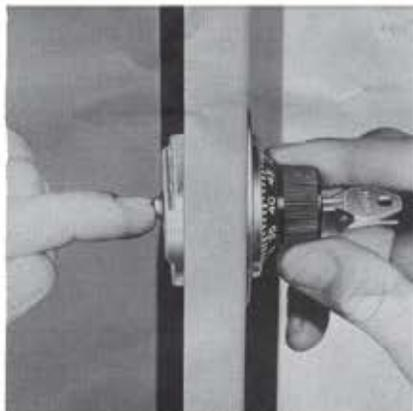
**4** With other hand, turn dial right to number 48. Do not turn dial more than two numbers with button depressed. Then release push-button.
