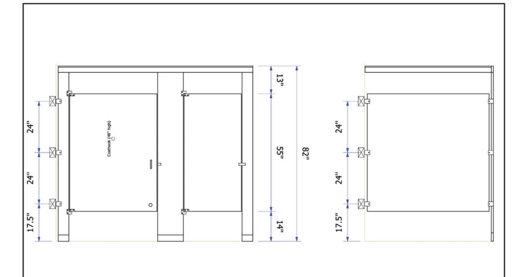
Material Texture: Pebble Grain (Std), Compartment Material Height: 55" High Doors/Panels - 14" AFF, Door Hardware: Vault Hinge & Slide Latch, Compartment Brackets: AL Stirrup (3/Connection), Trim Shoes: Stainless Steel, Door Thickness: 1.00", Pilaster Thickness: 1.00", Panel/Screen Thickness: 1.00"
