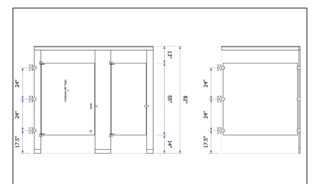
Material Texture: Pebble Grain (Std), Compartment Material Height: 55" High Doors/Panels - 14" AFF, Door Hardware: Vault Hinge & Slide Latch, Compartment Brackets: AL Stirrup (3/Connection), Trim Shoes: Stainless Steel, Door Thickness: 1.00", Pilaster Thickness: 1
