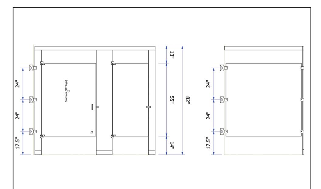
Material Texture: Pebble Grain (Std), Compartment Material Height: 55" High Doors/Panels - 14" AFF, Door Hardware: Vault Hinge & Slide Latch, Compartment Brackets: AL Stirrup (3/Connection), Trim Shoes: Stainless Steel, Door Thickness: 1.00", Pilaster Thickness: 1.00", Panel/Screen Thickness: 1.00"
