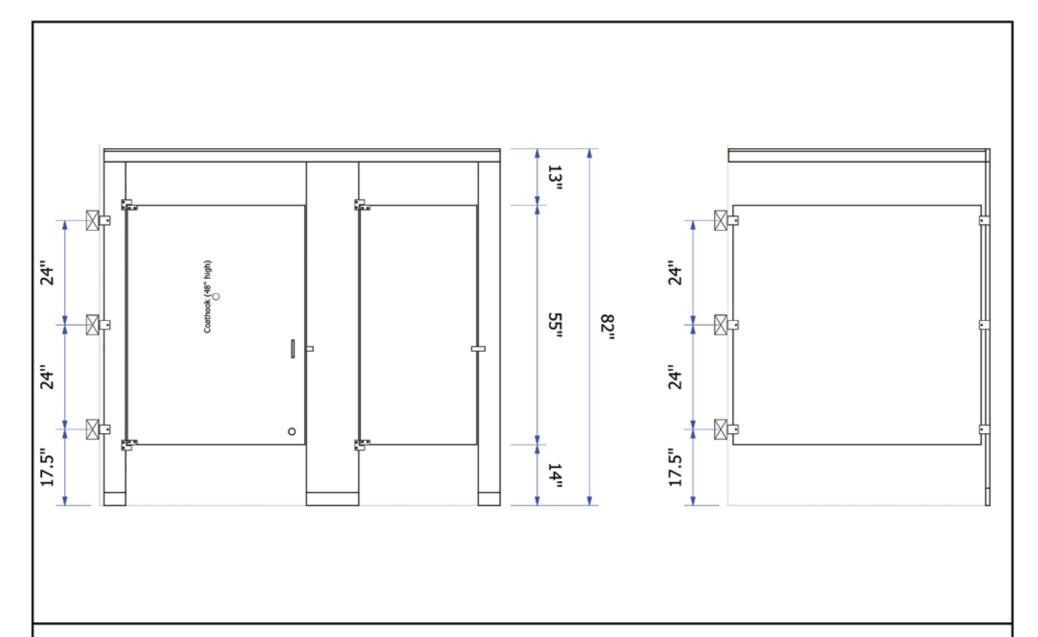
Material Texture: Pebble Grain (Std), Compartment Material Height: 55" High Doors/Panels - 14" AFF, Door Hardware: Vault Hinge & Slide Latch, Compartment Brackets: AL Stirrup (3/Connection), Trim Shoes: Stainless Steel, Door Thickness: 1.00", Pilaster Thickness: 1.00", Panel/Screen Thickness: 1.00"
