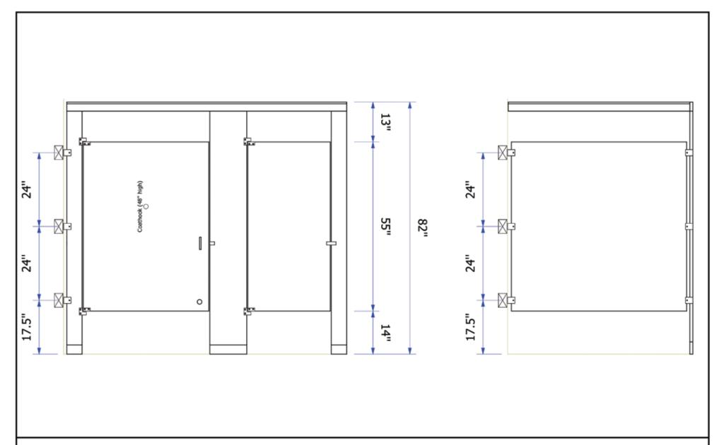
Material Texture: Pebble Grain (Std), Compartment Material Height: 55" High Doors/Panels - 14" AFF, Door Hardware: Vault Hinge & Slide Latch, Compartment Brackets: AL Stirrup (3/Connection), Trim Shoes: Stainless Steel, Door Thickness: 1.00", Pilaster Thickness: 1
