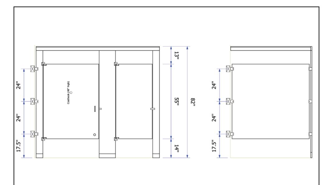
Material Texture: Pebble Grain (Std), Compartment Material Height: 55" High Doors/Panels - 14" AFF, Door Hardware: Vault Hinge & Slide Latch, Compartment Brackets: AL Stirrup (3/Connection), Trim Shoes: Stainless Steel, Door Thickness: 1.00", Pilaster Thickness: 1
