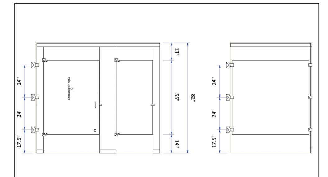
Material Texture: Pebble Grain (Std), Compartment Material Height: 55" High Doors/Panels - 14" AFF, Door Hardware: Vault Hinge & Slide Latch, Compartment Brackets: AL Stirrup (3/Connection), Trim Shoes: Stainless Steel, Door Thickness: 1.00", Pilaster Thickness: 1.00", Panel/Screen Thickness: 1.00"
