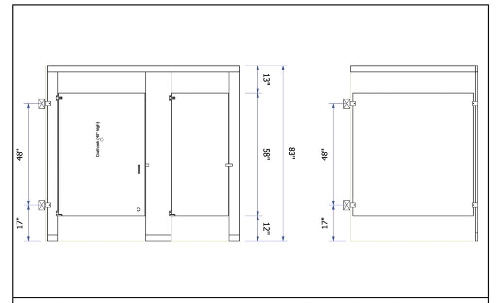
Compartment Material Height: 58" High Doors/Panels - 12" AFF, Door Hardware: Standard Chrome Hinge & Concealed Latch, Compartment Brackets: Chrome Stirrup, Trim Shoes: Stainless Steel, Door Thickness: 1.00", Pilaster Thickness: 1.25", Panel/Screen Thickness: 1.00"
