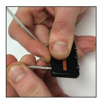
**Step 1:** On the top of your locking mechanism you will see a small button on the top. Press the button to release the cable from the lock. To reset your combination, keep the button firmly pressed down
